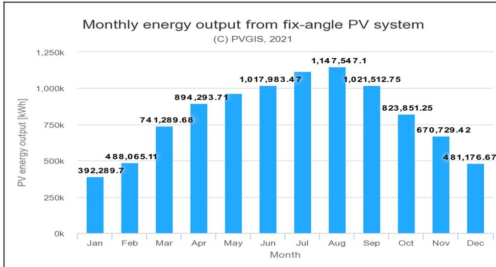
Figure 6. Monthly electrical energy production data of the last SPP with an installed capacity of 6750 MW [14]
