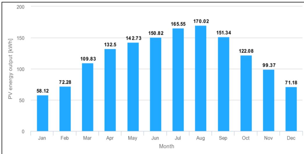
Figure 5. SPP monthly electricity energy generation belonging to YOBU location (kWh/m<sup>2</sup>) [14]
