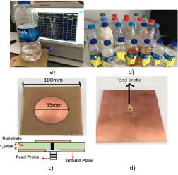
Figure 1. a) Measurement system used in this study b) Samples c) The geometry and front view of the patch antenna d) Back view of the patch antenna.
