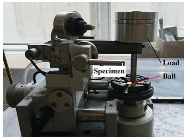
**Figure 4. Ball-on-disc wear testing machine**
