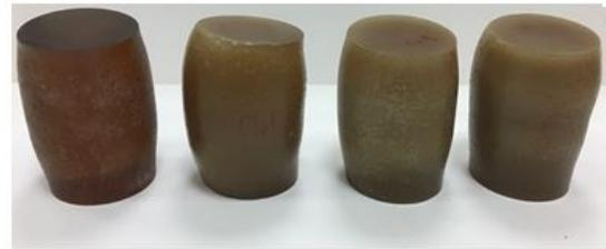
**Figure 8:** Tincal-reinforced composite specimens after compression strength test.
