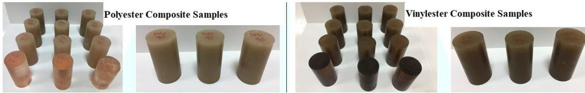
**Figure 2:** Tincal-reinforced composite samples before and after compressive strength test.
