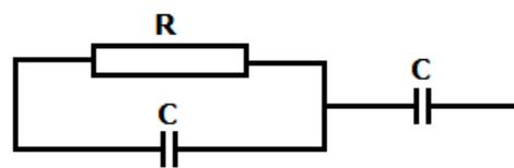
**Figure 11:** Tincal reinforced resin composites equivalent circuit diagram.
