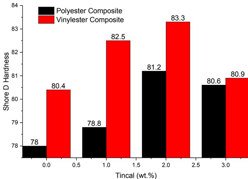
**Figure 7:** Shore D hardness values of tincal reinforced resin composites.
