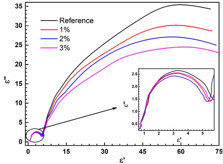
**Figure 10:** Cole-Cole diagram of tincal reinforced vinylester composites.
