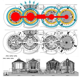
**Figure 3.** Ground floor plan and longitudinal section; plan and section drawings illustrating the spatial uses and the horizontal to vertical relationship of the Gasometer structures (www.gasometer.org, June 2005).
